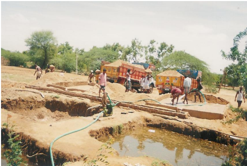
Fig 2: Sand being washed using compressor pump to remove red sting as white color sand fetches high price, Gauribidanur taluk, Karnataka, 2003
